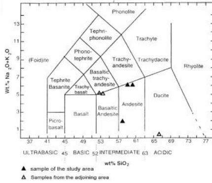
Figure (2) The chemical classification of the Mawgyi andesite based on total alkalis ( $\text{Na}_2\text{O}+\text{K}_2\text{O}$ ) and silica ( $\text{SiO}_2$ ), (Le Bas et al, 1996)
